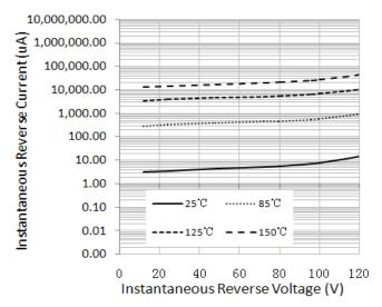
Figure 3. Typical Reverse Characteristics
