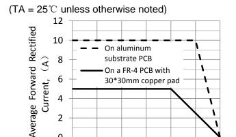
Lead temperature ( $^{\circ}$ C) Figure 1. Forward Current Derating Curve
