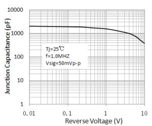
Figure 5. Typical Junction Capacitance
